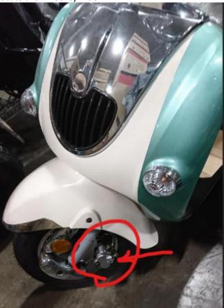
The wheel cylinder is on the left side of the scooter. Find it.
