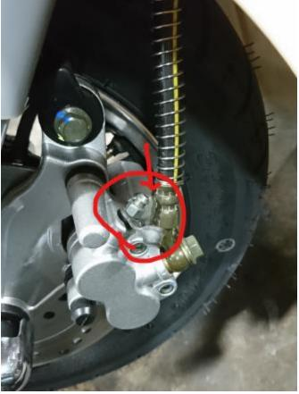
There is a vent valve with the wheel cylinder. Loose it.
