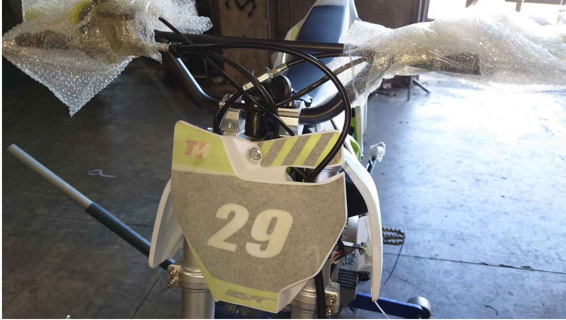
Figure 2.12.: Install the Number Plate
