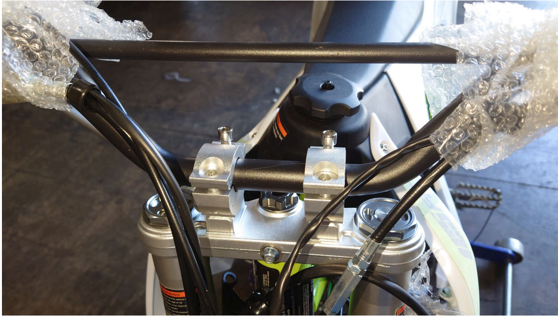
Figure 2.6.: Semi-Install the Handlebar Clamps
