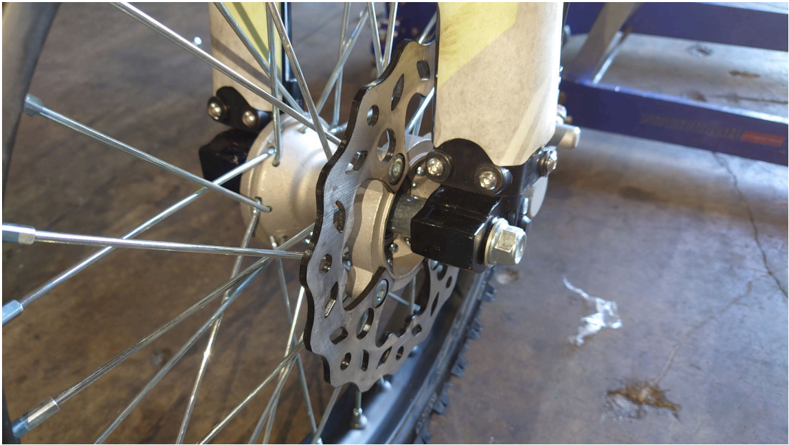
Figure 2.11.: Align the Brake Disc and Fasten the Nut
