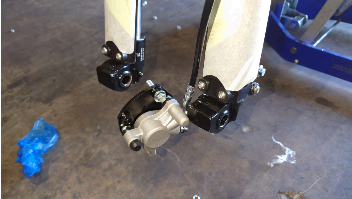
Figure 2.8.: Un-install the Front Caliper and Remove the Buffer Pad
