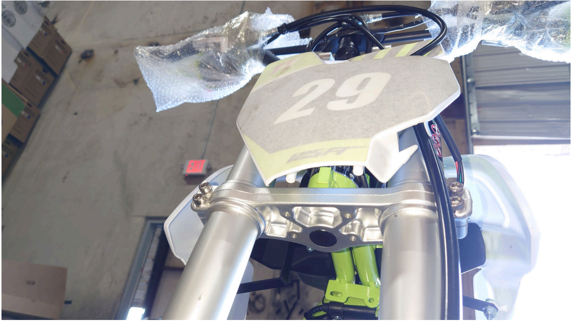
Figure 2.13.: Take off the Screws underneath the Triple Tree Clamp
