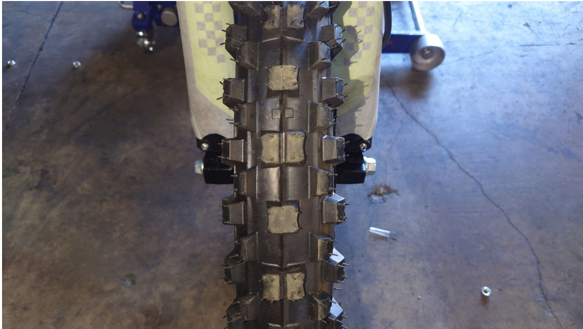
Figure 2.10.: Put on the Front Wheel and Front Axle
