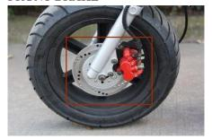
Please check the fluid lever whether it is upward the "LOWER" level mark
