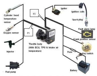
Figure I. EFI system configuration diagram
