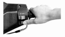
• Press down starter switch button to use electric starter:
