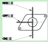
This type of motorcycle is equipped with manual acting fuel cock. There are three positions: "ON", "RES" and "OFF".
