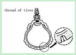
It is dangerous to use the wear tires; it will affect the traction, stability, steering and operating system. A new front tire should be replaced when the depth of thread is decreased below 1.6 mm.
