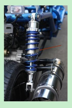
There is shock absorber in the front the rear wheel; it is designed according to rider's requirements, loading, road condition and other factors. It is factory set and no adjustment is needed.
