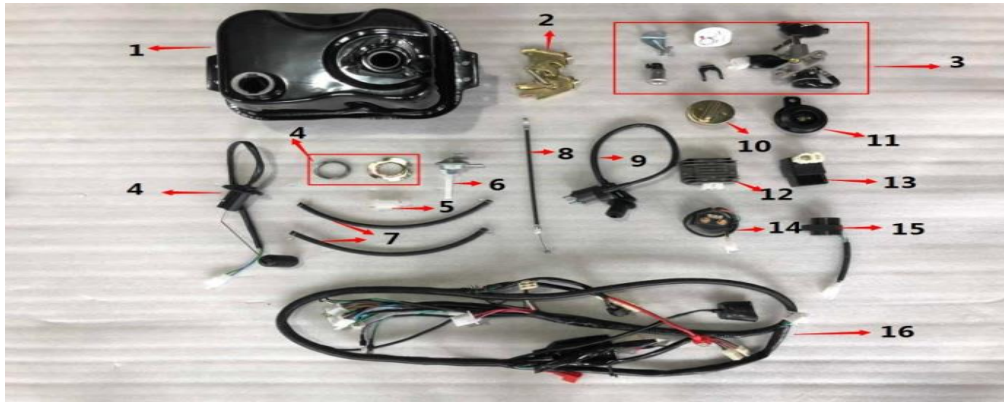
Figure: H:fuel tank, igniter, etc(图H: 油箱、点火器等)
