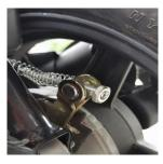
Brake adjusting Nut cap
