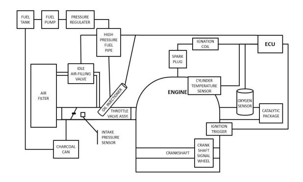
As shown in the figure, the motorcycle EFI system mainly includes ECU, oil supply system, ignition system, throttle & intake tube assembly, crankshaft signal system, cylinder temperature sensor, intake pressure sensor, oxygen sensor (optional) and wire beam. Among them, the throttle valve and intake pipe assembly include the throttle valve body, TPS (optional), MAP & idle filling valve.
