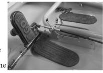
pedals and make sure you are getting a good pulling from the cable it seft. Once you are satisfied with the adjustment, secure all nuts to complete the adjustment.
