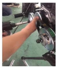
F) Tighten the M16x1.5self-locking nut on the driven pulley with
