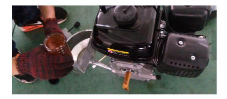
5. Install the clutch jackshaft plate 58200-L: (note: if your mini bike comes with pre-assembled engine, you may skip this step), attach the jackshaft 58200-L on the engine using M8x16 bolt, please do not tighten all the bolts at this step.
