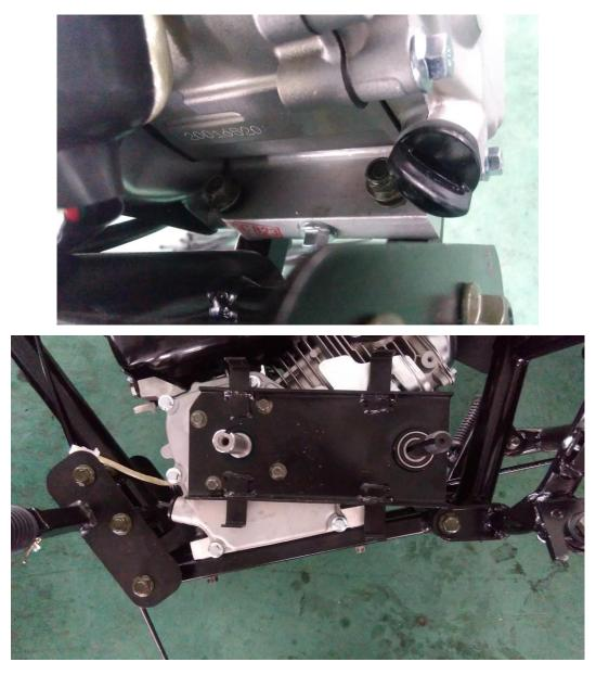
7. Install the flat key and 10 teeth sprocket (note: if your mini bike comes with pre-assembled engine, you may skip this step)
