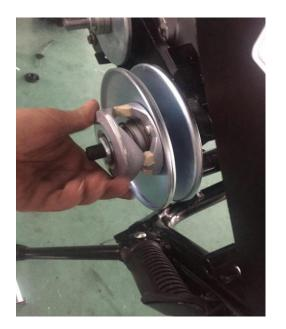
B) Put 12.5mm bushing, 1pc of 3.5mmwahser and 4pc of 1mm washer in turn onto the engine output shaft (remark: the reason to have the washers is to make the alignment of front clutch to the rear driven pulley, so you may need change the quantity of the washers you put in there)
