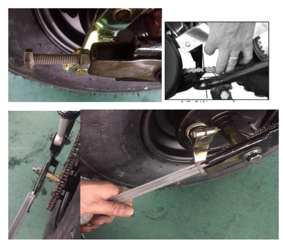
C) Tighten the adjuster bolt
