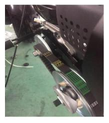
E) Install the front clutch bushing, front clutch cover. Tighten the M8x55 bolt with torque 22-29Nm
