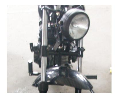
3. Install the front wheel: determinate the rotate direction of the front wheel, install it with the front wheel axle M14\*1.5\*310 and the self-locking nut M14\*1.5. The requested torque is 56-62N.m.
