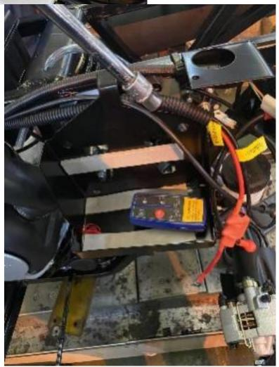
步骤六:将绞盘开关安装到左侧龙头把手上(走线需要将前面塑料盖板拆除) 6. Install the winch switch to the left side of the handle bar by removing the handle bar
