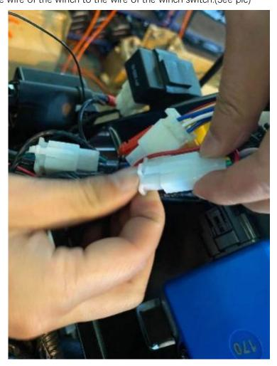
步骤八:将绞盘开关上的红线,与车子主电缆上的端子对插(每台车上都有此端子) 8. Connect the red wire of the winch switch to the terminal of ATV wire harness. (See pic). The wire harness of each ATV has the terminal to connect.
