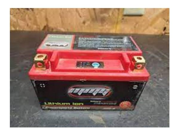
Check the battery and make sure it is charged and properly connected. Charge or replace the battery if necessary. Please note that both AutoZone and O'Reilly Auto Parts offer free battery volt and amp testing upon request. We also recommend trickle charging the battery for at least 8 hours before it's initial use to extend the longevity of your battery's life.
