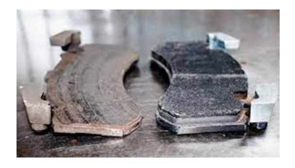
Check the brake pads and make sure they are not worn down. Replace the brake pads if necessary.
