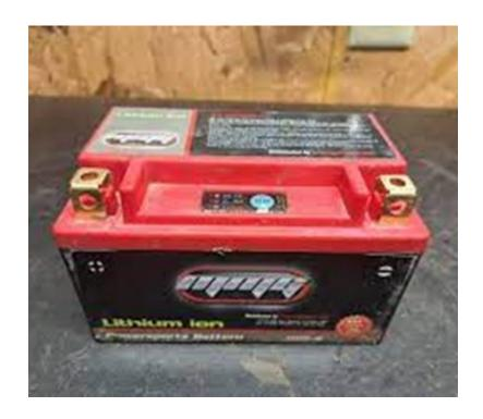
Check the battery and make sure it is charged and properly connected. Charge or replace the battery if necessary. Please note that both AutoZone and O'Reilly Auto Parts offer free battery volt and amp testing upon request. We also recommend trickle charging the battery for at least 8 hours before it's initial use to extend the longevity of your battery's life.
