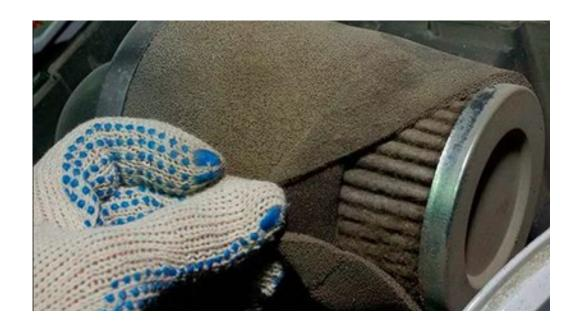
Check the air filter and clean or replace it if necessary.
