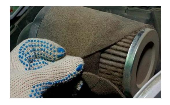
Check the air filter and clean or replace it if necessary.
