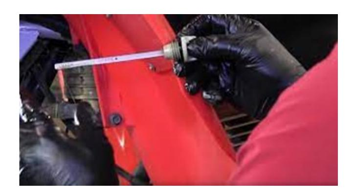
Check the transmission fluid level and make sure it is topped off.
