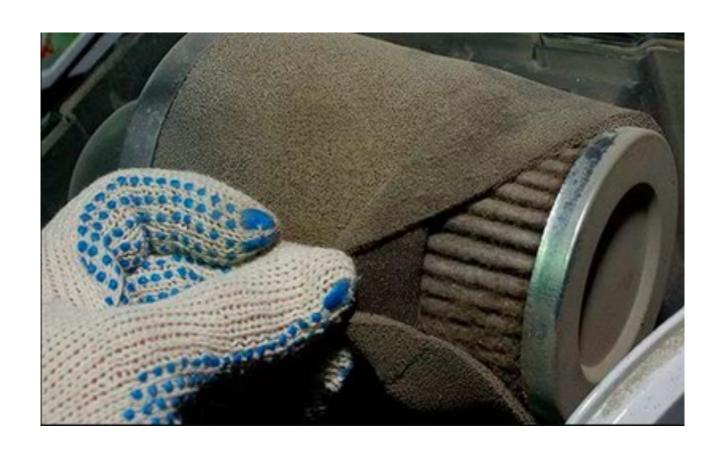
Check the air filter and clean or replace it if necessary.
