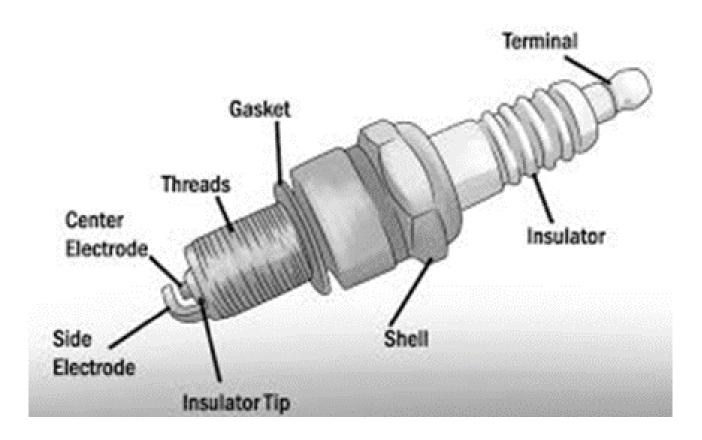
Check the spark plug and make sure it is clean and properly gapped.
