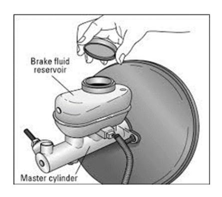
Check the brake fluid level and make sure it is topped off. Refill the brake fluid if necessary.
