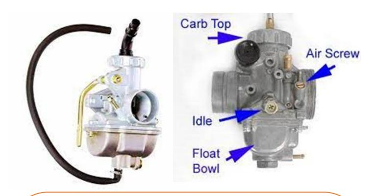
Check the carburetor and make sure it is clean and functioning properly.
