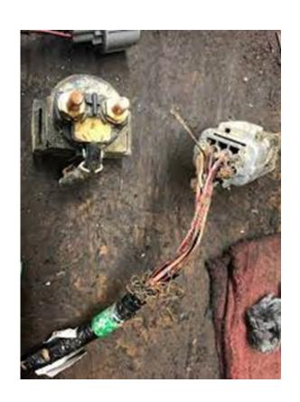
Check the wiring connections and make sure they are not loose or corroded. Clean or replace any damaged connections.
