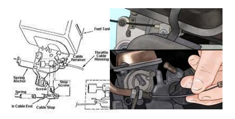
Check the throttle cable and make sure it is properly adjusted.
