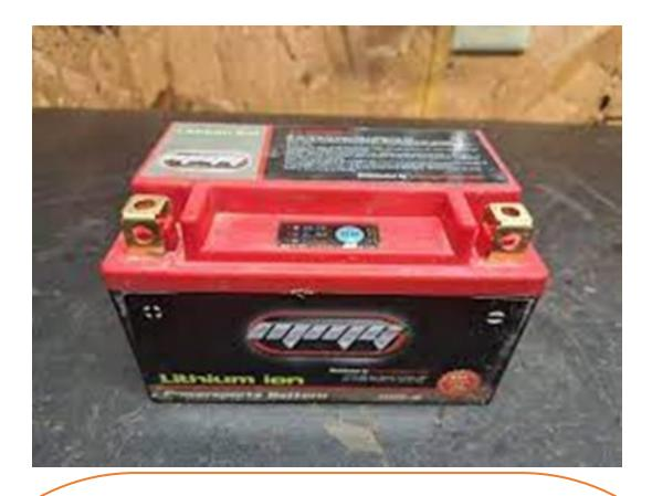
Check the battery and make sure it is charged and properly connected. Charge or replace the battery if necessary. Please note that both AutoZone and O'Reilly Auto Parts offer free battery volt and amp testing upon request (ensure
