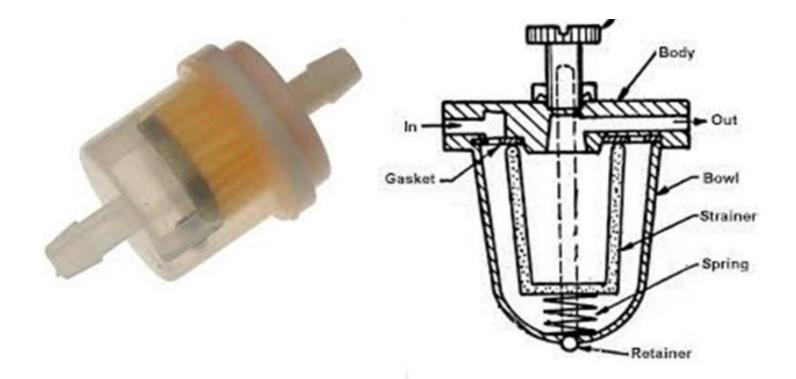
Check the fuel filter and make sure it is clean and not clogged.
