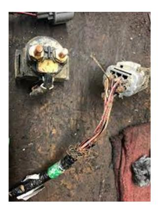
Check the wiring connections and make sure they are not loose or corroded. Clean or replace any damaged connections.
