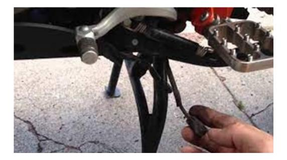
Check the kickstand switch and make sure it is functioning properly. If the switch is faulty, replace it.
