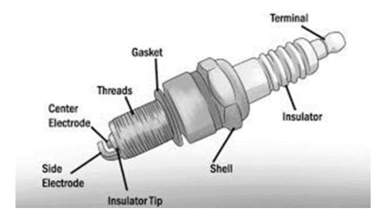
Check the spark plug and make sure it is clean and properly gapped. Replace or clean the spark plug
