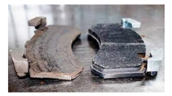
Check the brake pads and make sure they are not worn down. Replace the brake pads if necessary.
