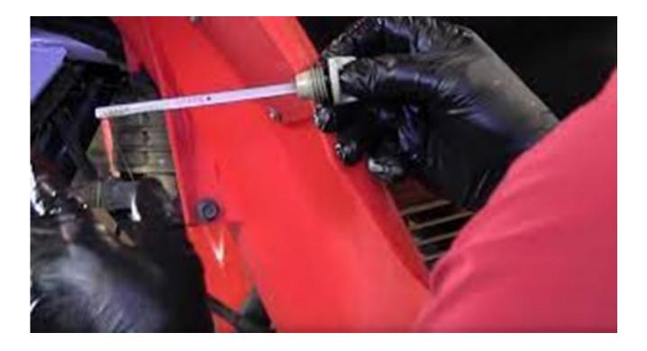
Check the transmission fluid level and make sure it is topped off (if applicable/has second transmission unit)
