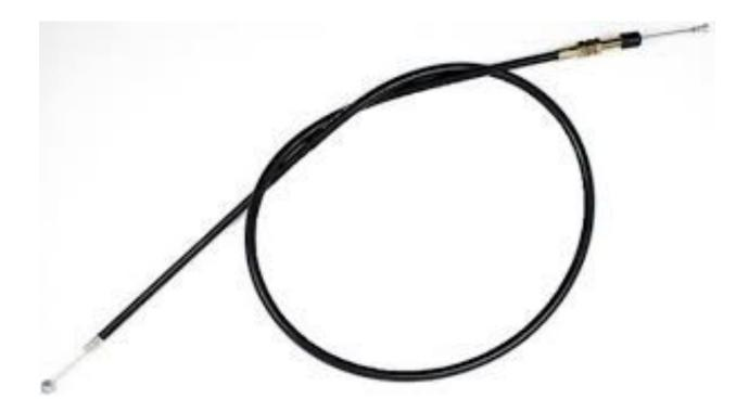
Check the clutch cable and make sure it is properly adjusted. Adjust the cable if necessary.
