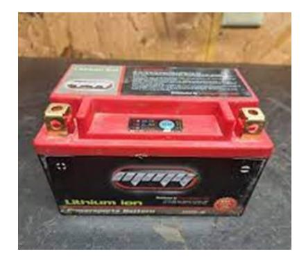
Check the battery and make sure it is charged and properly connected. Charge or replace the battery if necessary. Please note that both AutoZone and O'Reilly Auto Parts offer free battery volt and amp testing upon request (ensure
