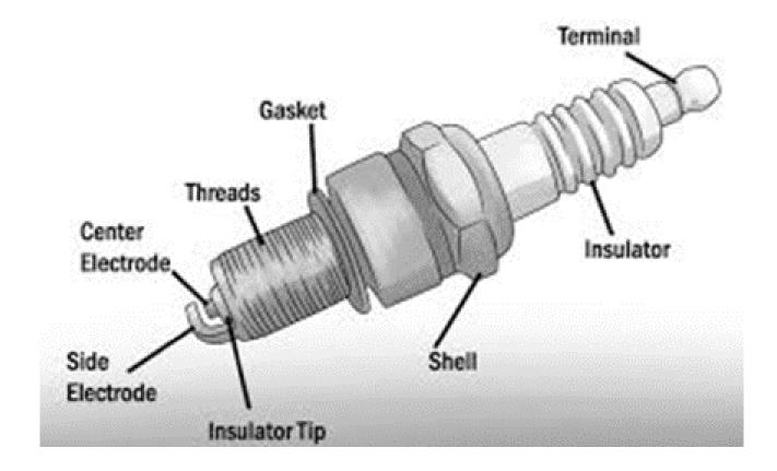
Check the spark plug and make sure it is clean and properly gapped.
