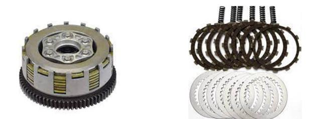
Check the clutch plates and make sure they are not worn or damaged. Replace the plates if necessary.
