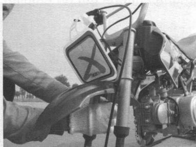
7、Install front fender
