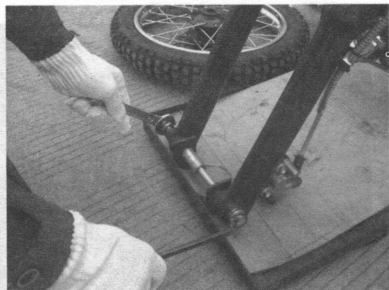
7、Loosen front shock absorber fixer
