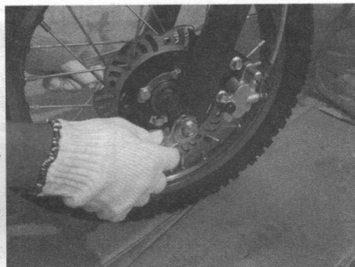
8、Install front wheel
