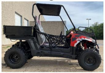
The TrailMaster Challenger 200U with a 169cc GY6 engine is a new model with a Large 27.5"X45.3"X93.5" dump bed with max load 165lbs, flips down 32 degrees. This aggressive Challenger has a new gear ratio set up which offers maximum low-end torque.
