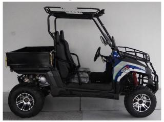
The TrailMaster Challenger 200EUX with an electronic fuel injected (EFI) 11.1 hp 169cc GY6 engine with internal F N R transmission is a new model with a Large 27.5"X45.3"X93.5" dump bed with max load 165lbs, flips down 32 degrees. This aggressive Challenger has a new gear ratio set up which offers maximum low-end torque with a top speed of 38mph
