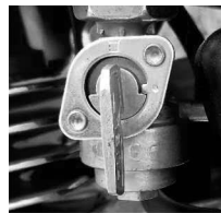
Fuel Valve ON
