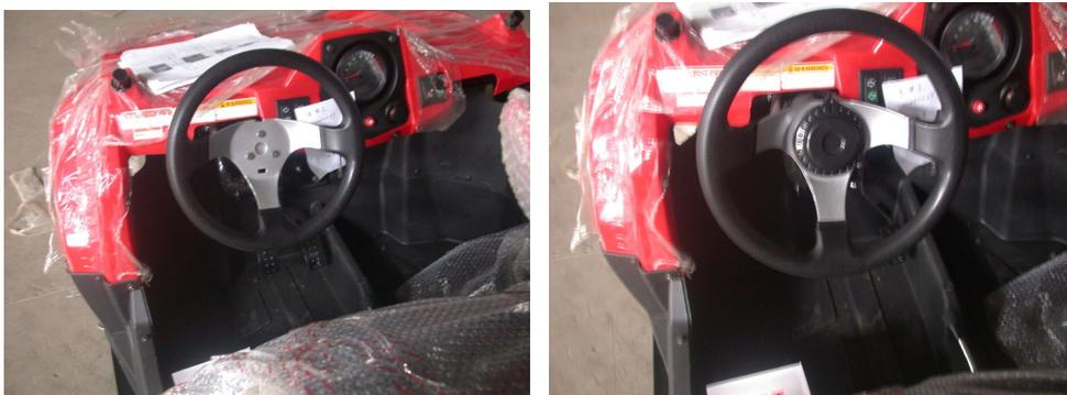
2.10 Adjust the steering wheel angle: loose the adjustment nut as shown in the picture, adjust the steering wheel to a comfortable height, tighten
