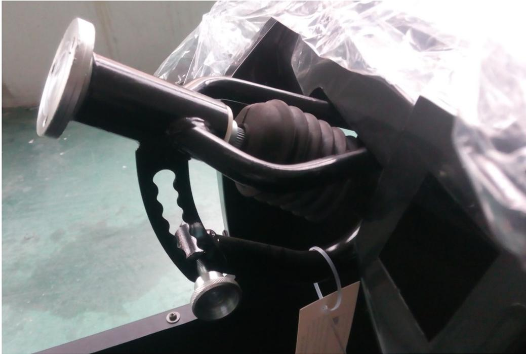
2.11 Install the front roll cage bar: put the front roll cage bar into the mount posts on the frame, put in the M8x60 bolt, R-washer, windshield bracket and tighten the M8 nut to fix.
