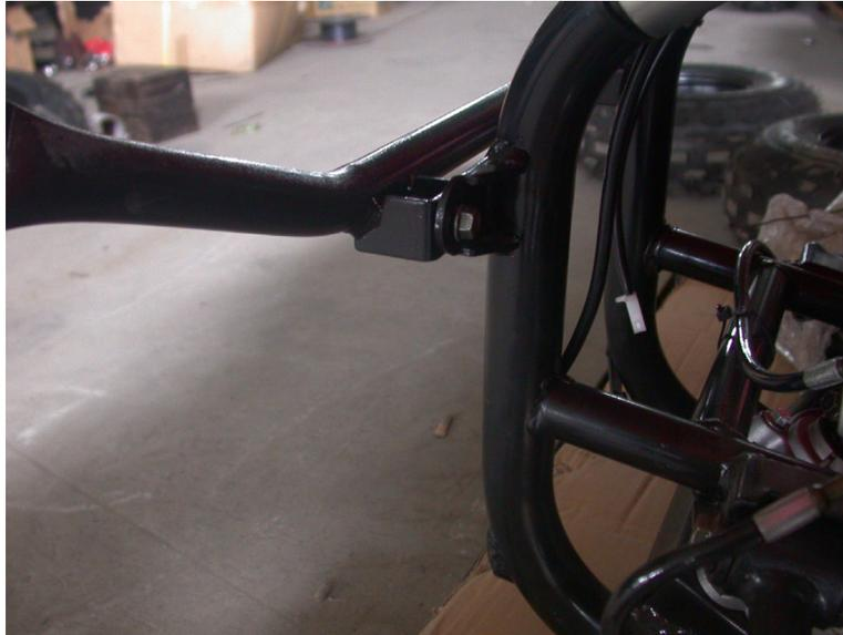
2.6 Set up the top headlights wire: open the right side of front hood cover as displayed in the picture, put the wire through the hole on the front hood cover where the front roll cage bar mount rod is, connect the plugs
