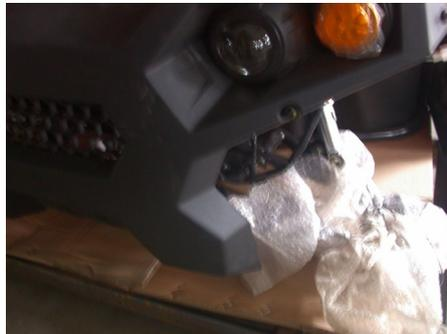
2.8 Plug the headlight and turn lights' wire: plug the wires with the connecting sockets; tighten the wires using zip ties.
