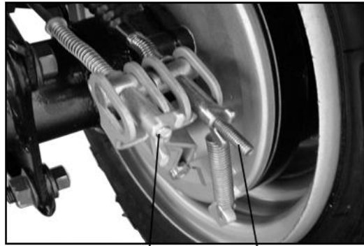
Brake rod adjustment nut (foot brake)
