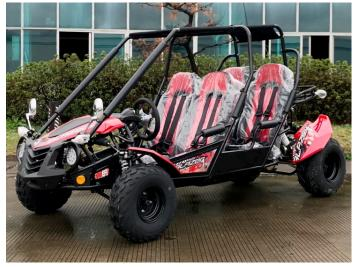
The TrailMaster Blazer4 200EX is an upgrade from the Blazer4 150X, now with a bigger 169cc GY6 engine and equipped with EFI. With fuel injection, users don't need to worry about starting in cold weather or at high altitudes; Furthermore, users don't need to fix or replace carburetors after periods of inactivity with the unit.
