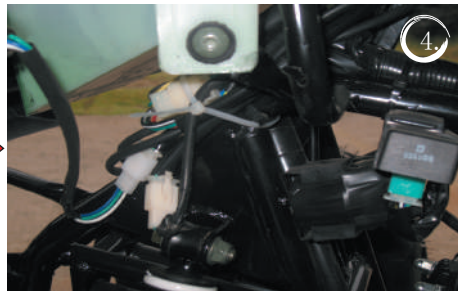
Fastening head light wire
