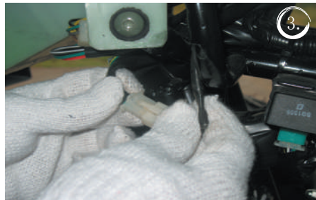
Connect head light wire
