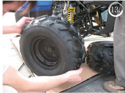
Install front wheel
