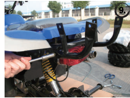
Install support of rear rack
