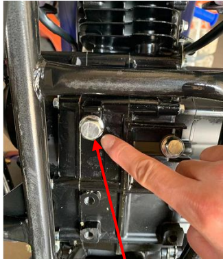
Engine oil drain bolt
