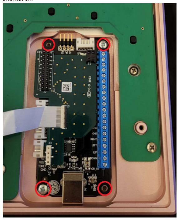
Step 6: Attaching the Ribbon Cable to the Main Board Attach the ribbon cable the same way as before (lifting the black tab from the back, sliding it in, and pushing the tab back down). Then, push down and crease the cable to keep it in place
