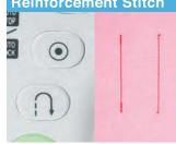
HZL-H series can sew a lock stitch at the beginning and end of sewing. There are two types of lock stitch, reverse stitch and reinforcement stitch.
