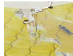
Transparent quilt presser foot makes the needle visible.
