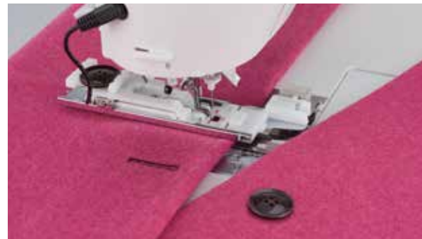
Buttonhole sewing with clamping plate and sensor
