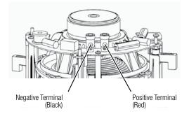
Press down on the post to open the hole; insert the bare end of the wire into the hole and release the post to secure the wire.
