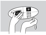
3. Cut the ceiling drywall along the mark you made in Step 2 to create the mounting opening.
