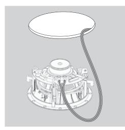
5. Attach the speaker's seismic tab to a support line, as per local safety regulations.
