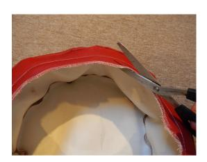
Most 6" Speakers will required no trimming of the hood. For larger speakers, trim flange to fit. For most 8" speakers, trim just inside the stitching. If your speaker needs to be installed close to a joist, you can offset the hole by cutting past the stritching to create an oval shaped opening.
