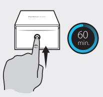
30 seconds before starting, the blue LED goes on standby. Open and close the lid again to start the cycle by pressing the touch button.
