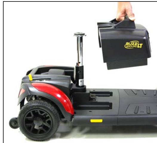
Figure 15. Removing the Battery Pack
