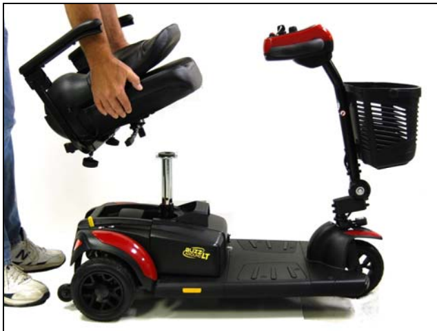
Figure 14. Removing the Seat
