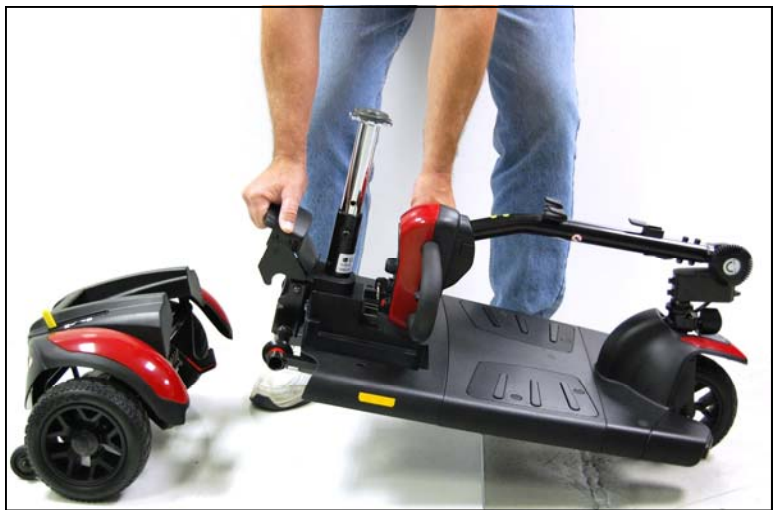
Figure 20. Connecting Frame and Drivetrain
