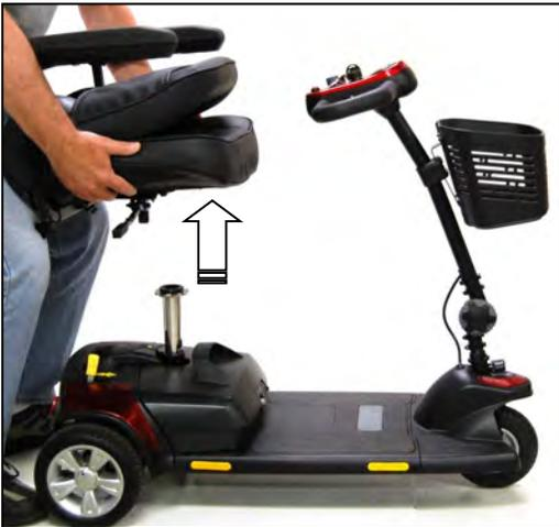
*Figure 14. Removing the Seat*
