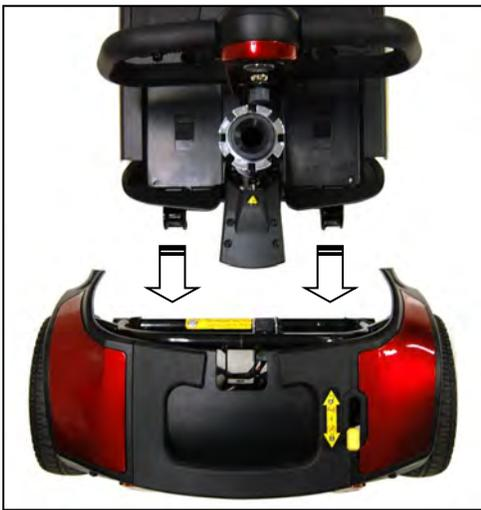
**Figure 19. Drivetrain Alignment**
