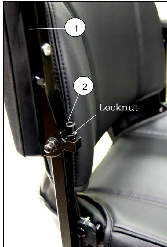
**Figure 7. Armrest Angle Adjustment**
