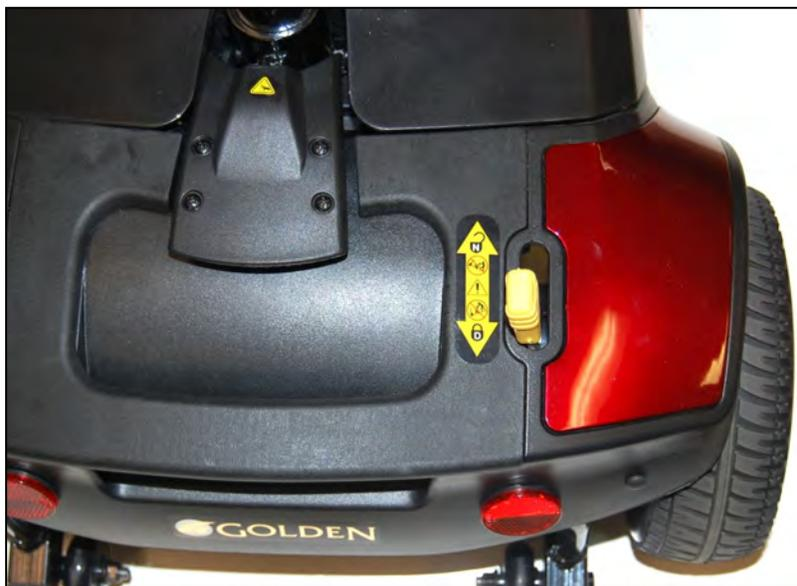
**Figure 11: Freewheel Lever (Drive Position)**
