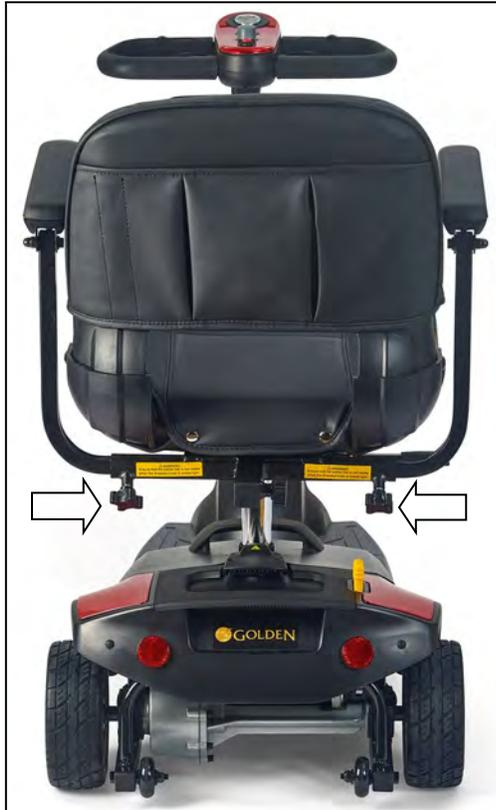
**Figure 6. Armrest Width Adjustment**
