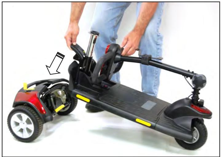
**Figure 20. Connecting Frame and Drivetrain**
