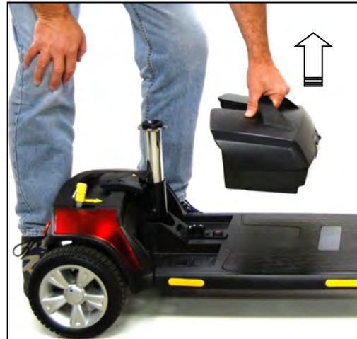
*Figure 15. Removing the Battery Pack*
