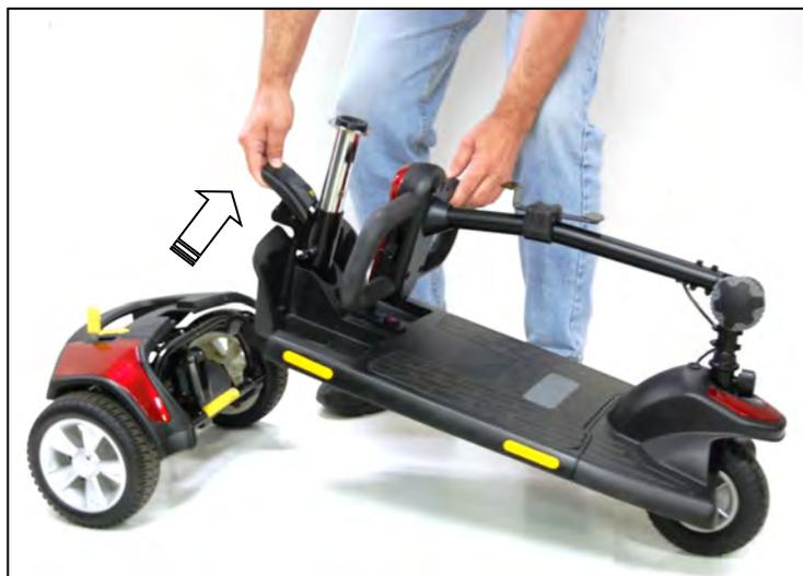
**Figure 17. Separating the Drivetrain and Frame**
