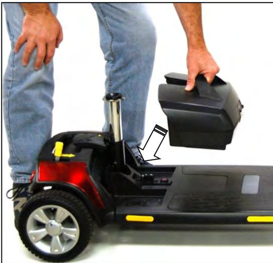
**Figure 21. Battery Pack Installation**
