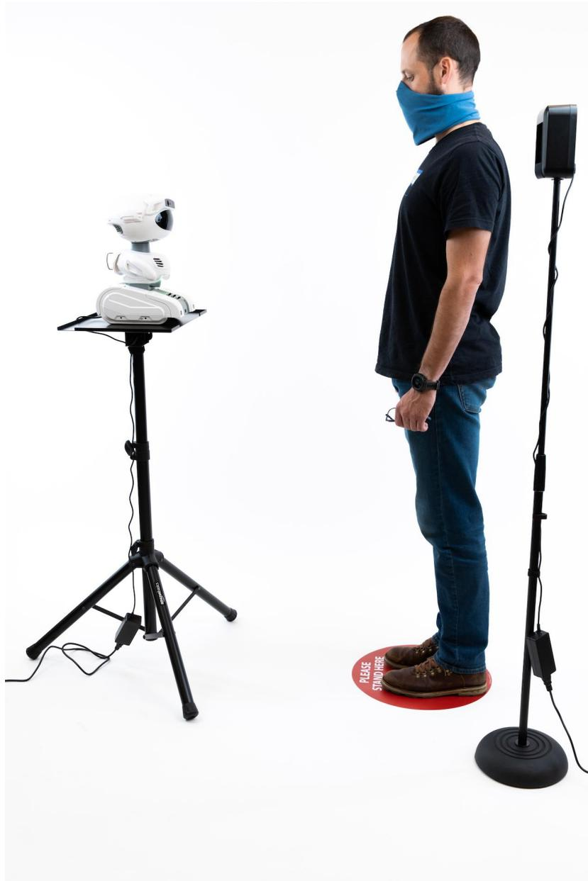
*Temperature Reference device incorrectly aligned, it is not in the same plane as the person being screened*
