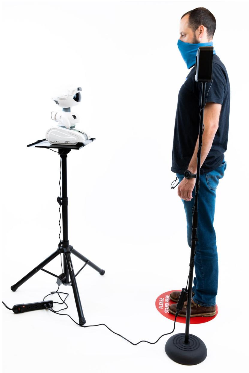
*Temperature Reference device correctly aligned*
