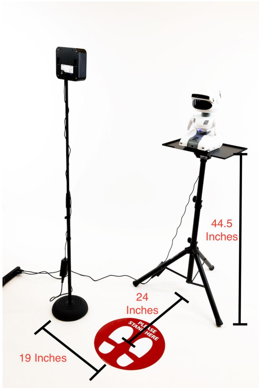
*19 inches from the center of the Temperature Reference Device to the Center of the please stand here mat*
