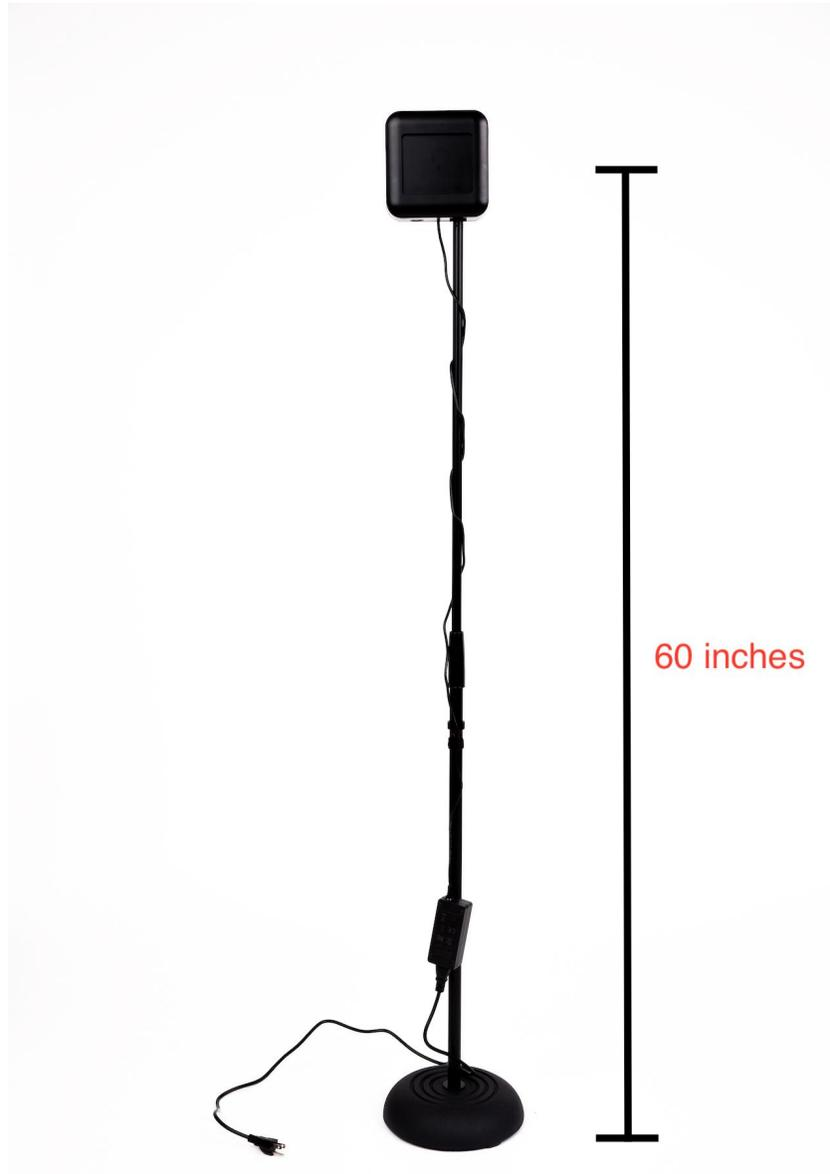
*60 inches from floor to middle of the Temperature Reference Device*
