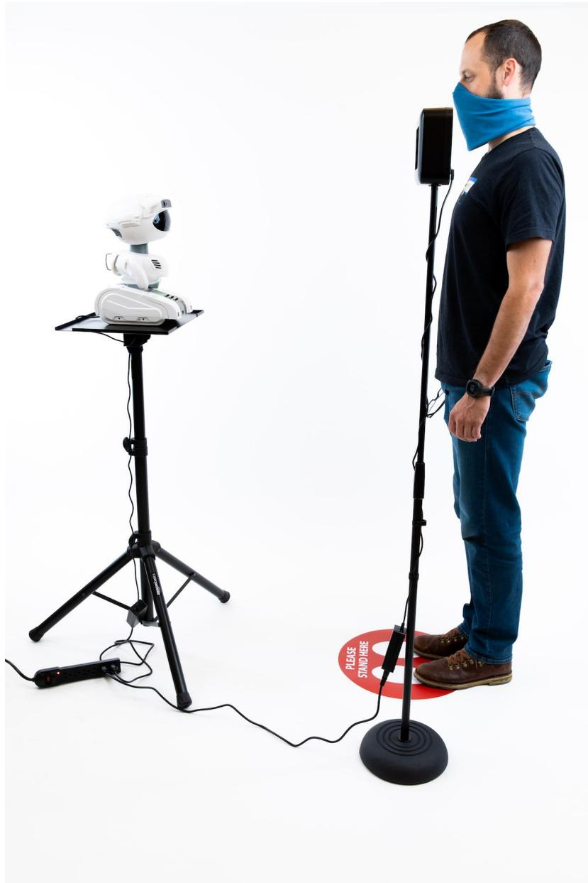
*A person not standing correctly on the mat causing the misalignment of the Temperature Reference Device during the screening*
