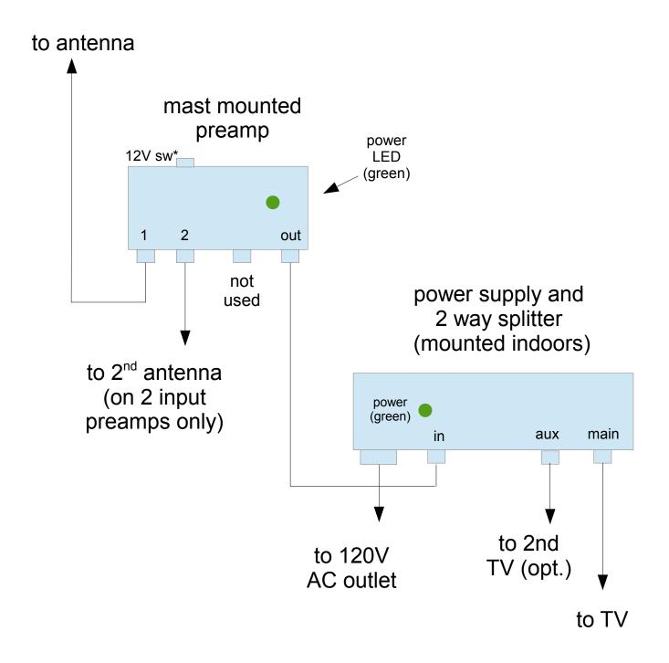
install preamp with the connectors / cables facing down as shown, to keep rain out
