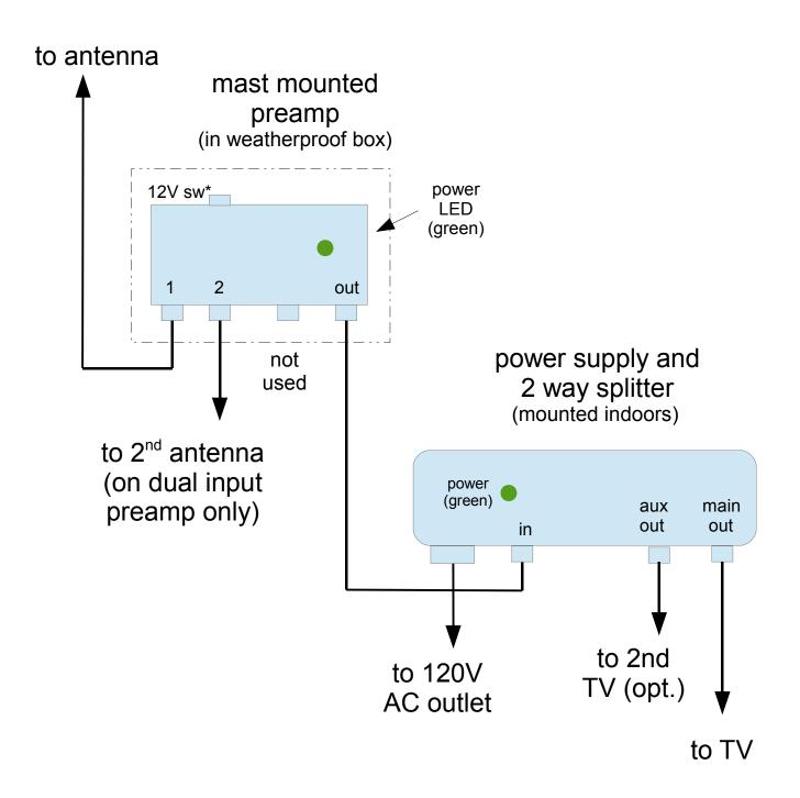
to keep rain out, install preamp with the connectors / cables facing down as shown
