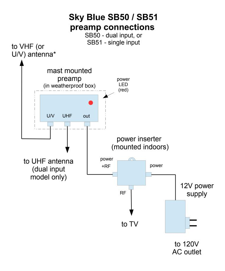
\*combo link switch (SB50 only): ON – single antenna on U/V input (antenna can be UHF, VHF or UHF+VHF) OFF – separate VHF and UHF antennas
