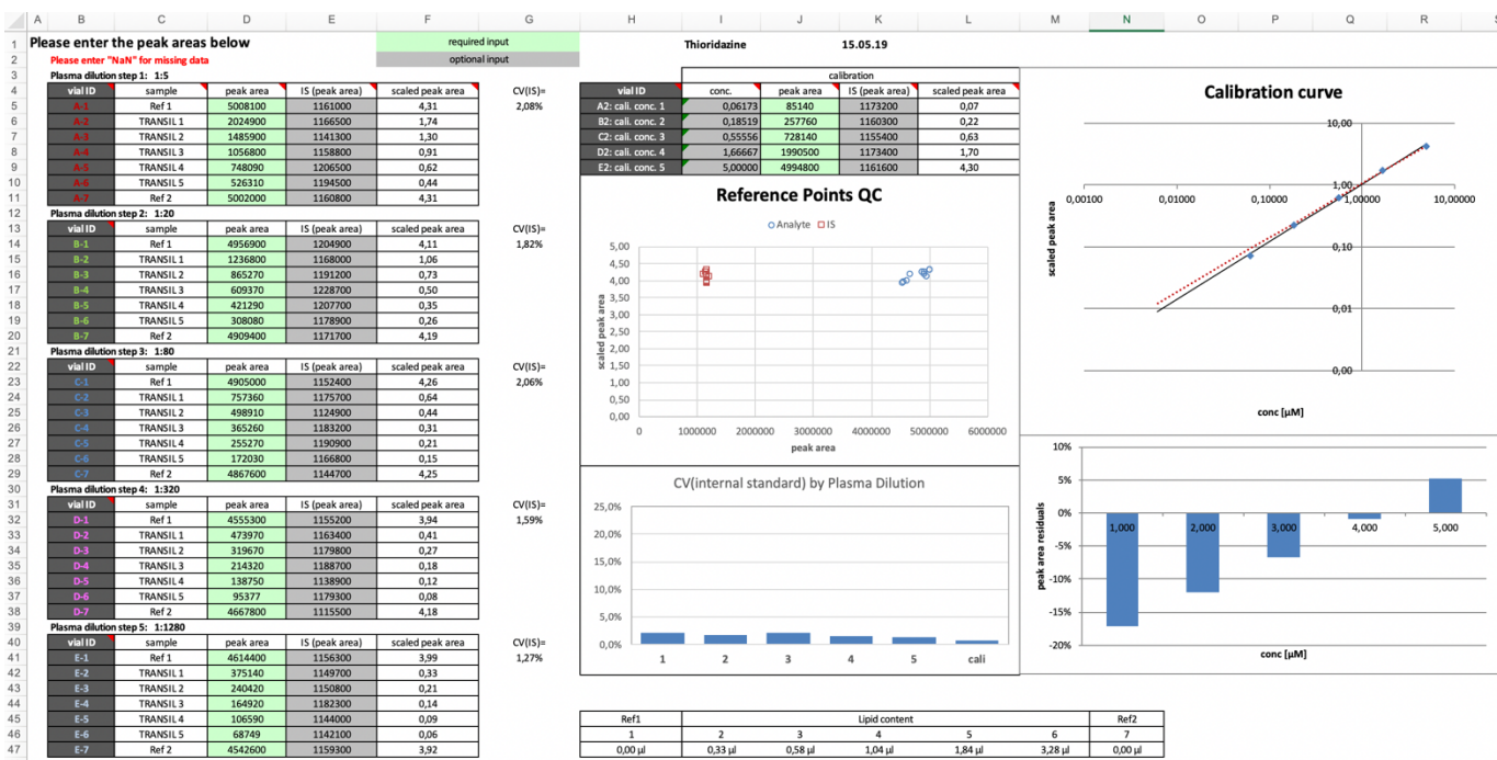
Figure 8: Screen shot of the spreadsheet’s “raw data” tab where quantification data need to be entered. The tab provides basic analysis of data quality. A calibration curve is shown that highlights the calibrations’ deviation from linearity (the instrument response is fully linear across the concentration range measured when the red dashed line aligns fully with the black regression line). The percentage deviation from linearity is shown in the bar chart below the calibration curve. The coefficient of variation of the internal standards is shown for all plasma dilutions and the calibration (lower left bar chart). And a plot of the scaled peak areas versus the peak areas highlights potential unwanted trends in the data such as instrument drift, that may adversely affect the results. The measurements should be inspected in more detail when the data points for the analyte and/or the internal standard are not clustered together, but have individual points in discrete locations.
