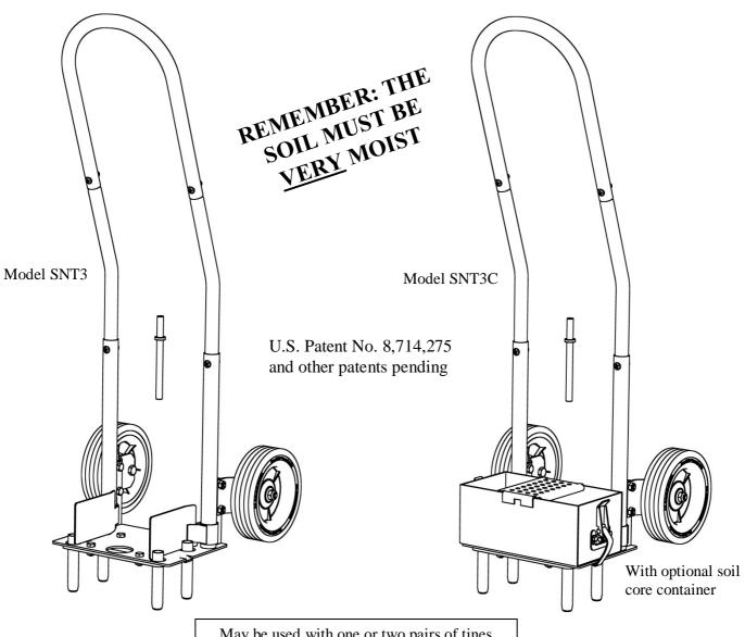
May be used with one or two pairs of tines Please begin by using one pair of tines only
