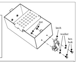
Step 5b: Place the container on a table or floor as shown below. Allow the latch body to slide down to its lowest position by gravity. Push the latch arm against the container. Make sure that latch arm is in contact with the edge and bottom of the container and the floor or table as shown. Tighten the bolts with your hand to temporarily secure the latches. Finally, tighten the bolts and nuts with 10mm wrenches.
