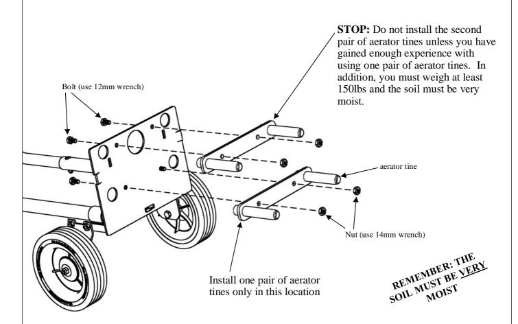
One pair of tines is intended for general purpose use. Two pairs of tines will require significantly more force to push the tines into the ground. It is intended for maintenance of healthy lawn only; it works well on grass with a very healthy root system only. Soil may stick to the spaces between the tines if the root system is poor.
