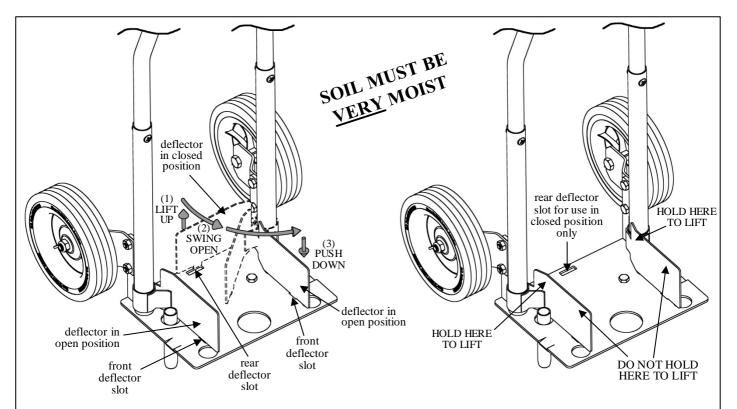
If you wish to leave the soil cores on the ground, adjust the deflectors to the open position as shown in the right picture above. To open a deflector, (1) lift the deflector up above the rear deflector slot, (2) swing the deflector open, and (3) push the deflector down to insert it into the front deflector slot as shown in the left picture above.
