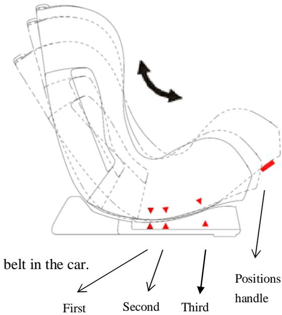
This car seat has three different backrest recline positions, it makes the baby feel more comfortable. The first and second positions are for the forward facing, the third position is for the rearward facing.
