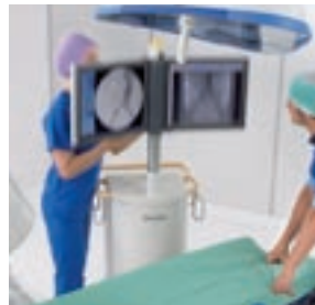
Height movement of the foldable monitors for optimal working and transport height.
