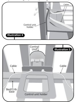
5. Pass the cords of the sensor pads through special openings in the holder (see illustration 4 and 5).
