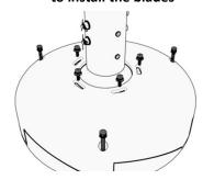
Remove the 5 inner screws followed by the 3 outer bolts to unsecure the motor cover. Lift and secure the motor cover with clamp to expose the motor assembly.
