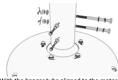
With the hanger tube aligned to the motor shaft, tighten the 2 bolts and 2 screws to secure the assembly. Install and expand the cotter pins.
