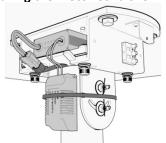
Insert the motor controller box into the fan mount. Secure the box using the double sided tape provided. Connect the wire harness to the terminal block.
