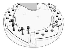
Unsecure the upper fan blade mount by removing the 4 bolts. Loosen the middle bolt. **DO NOT REMOVE THE LOWER FAN BLADE MOUNT!**
