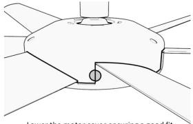
Lower the motor cover ensuring a good fit. NOTE THAT THE COLOUR POSITIONING MARKERS ARE TO BE ALIGNED.
