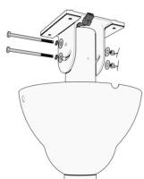
Ensure the canopy cover is inserted into the hanger tube before assembling the mounting bracket to the hanger tube.
