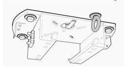
Mount the ceiling bracket using (4) 3/8" or equivalent lag screws . Install the closed eye bolt for safety cable. Ensure eye screw can be covered by the canopy cover.
