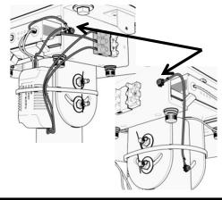
Connect the grounding wires to the ceiling bracket as shown.
