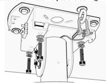
Lift the fan assembly and place it within the ceiling bracket. Secure fan using the bolts and washers provided.
