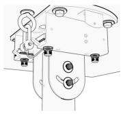
Adjust the hanger tube to be perpendicular to the ground. Fully tighten the 2 upper hanger tube bolts to secure the hanger tube.
