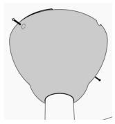
Raise the top canopy and secure it using the screws on both sides of the canopy..
