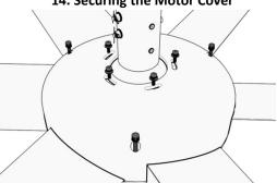
To secure the motor cover, insert and tighten the 3 outer bolts followed by the 5 inner screws. Rotate the fan by hand to check for problems. You are now ready to power up the fan.
