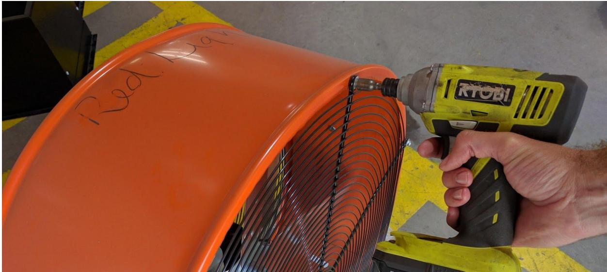
Remove the set screw that holds the fan blade in place on the motor shaft using a 5/16" box end wrench.
