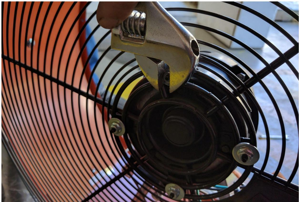
Replace the motor with the new XE420 ensuring that the threaded stud on the front of the motor is in the downward, or 6 o'clock, position.
