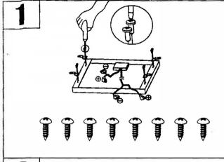
Mount the 4 brackets on the solar panel with the 8 screws provided.
