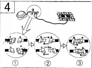
CONNECTING THE SOLAR PANEL: WARNING: Solar panels generate electricity when exposed to any light source; electrical shock and burns can result from direct contact with the panel terminals. Cover the panel surface with an opaque material before handling the electrical connections to the panel. Additional hazards exist whenever the panels are wet. Multiple solar panels may be used to increase the power/output on both the roof mount and gable attic vents.
