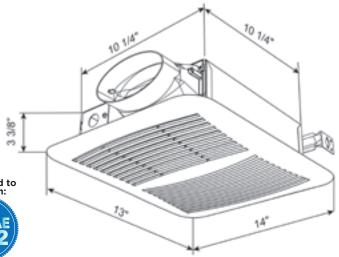
ETL Listed for use over bathtubs and showers when connected to a GFCI protected branch circuit (ceiling mount only).
