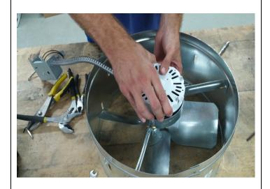
Tighten the three motor bracket bolts that were loosened in step 3.
