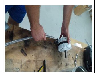
When the wires are out of the electrical conduit, remove the conduit from the thermostat box by turning the conduit counter clockwise. This will make it much easier when installing the new motor wires into the conduit.
