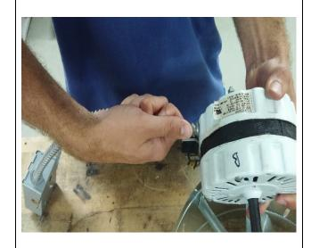
When the electrical conduit is removed from the motor pull the motor wires out of the conduit by pulling on the conduit and sliding it down the electrical wires.
