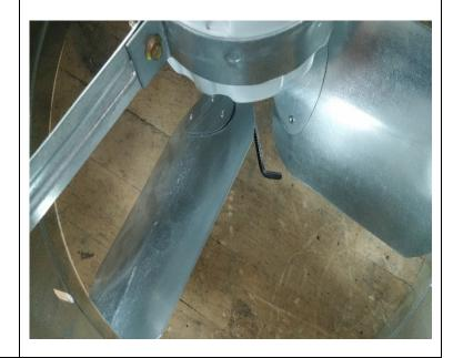
At this point spin the fan on the new motor to ensure that the fan is not rubbing anywhere.
