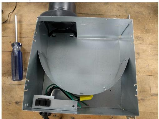
Step 4. When installing the new motor kit, note the tabs on the motor plate and the slots they correspond to in the housing. Also take care not to bend the mounting bracket the motor secures to on the motor plate during installation.
