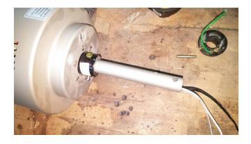
Step 3: With the rod loose from the motor, and with the end cap removed from the rod you can now slide the old rod down the length of wire and remove. You can now insert the wires into the new downrod. The motor has 4'6" of wire pre installed and by cutting 4' of downrod you will have 6" of wire left to connect to the power source.
