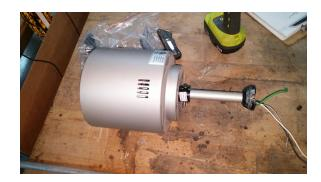
Step 1. Loosen two screws and pull the pin that is inside the mount. This will allow the end cap to come off the rod.
