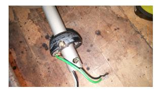
Step 2: On the motor end of the rod loosen the two screws and remove the cotter pin from the end of the keeper pin. This will allow the rod to be removed from the motor housing.
